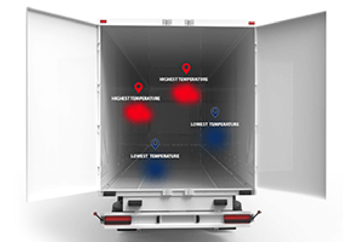
Figure A1.1 Example layout for monitoring a part loaded trailer
